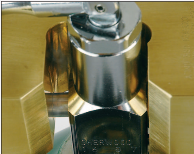
Figure 12. Valve is tight to the body.
