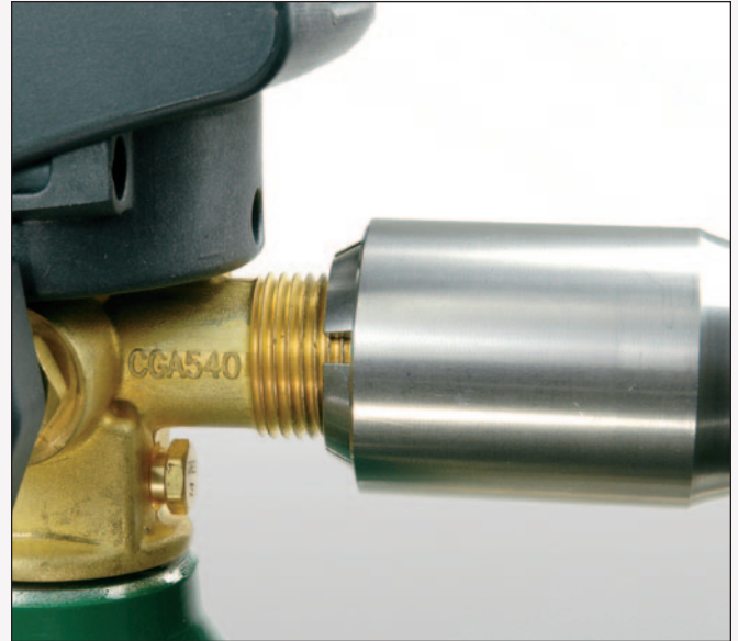
Figure 20. Note excess threads.
