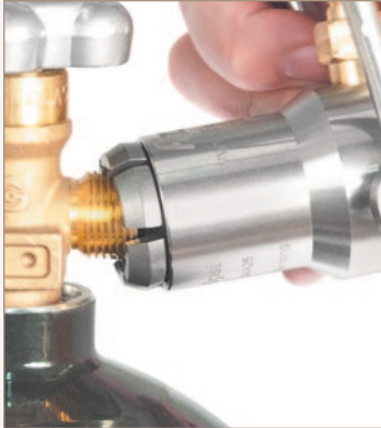
Figure 6c. Misaligned CGA 540/CGA 346
