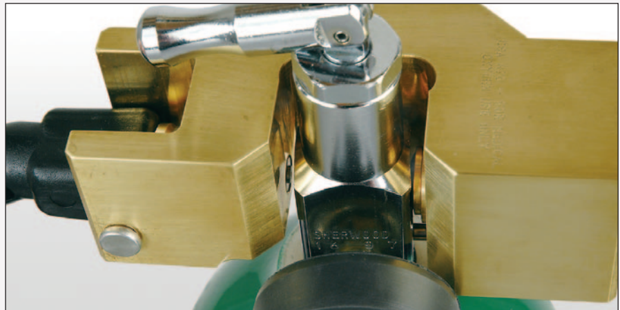
Figure 6 and 7. The piston retains position against valve during accidental disconnection.
