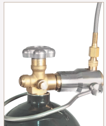
Figure 4c - 4d. Align the CGA 580 RPV tight and square against valve with no visible gap to avoid damage to the sealing surface
