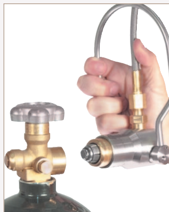
Figure 4c - 4d. Align the CGA 580 RPV tight and square against valve with no visible gap to avoid damage to the sealing surface
