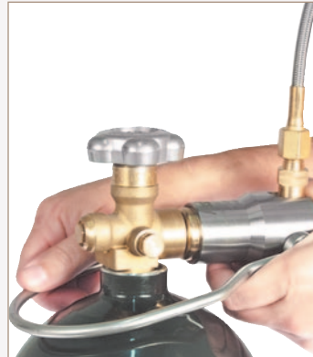
Figure 7a. Demonstrates good connection using CGA580/580 RPV
