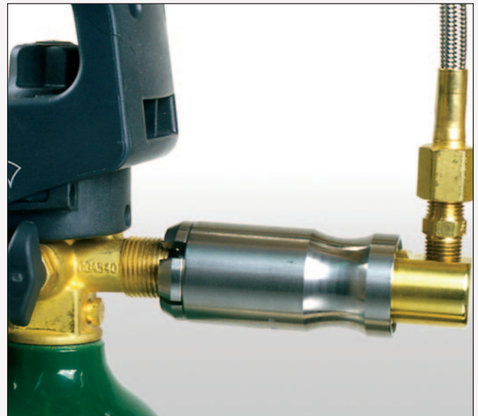
Figure 21. Connector loose. Sleeve not forward.
