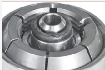
Figure 12. An example of a bad O-ring main seal
