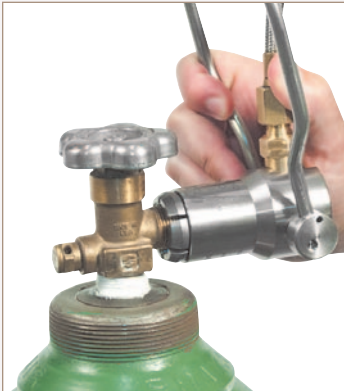
Figure 6a. Use minimal force on bail
