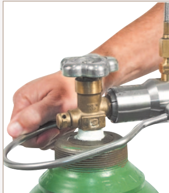
Figure 6b. Demonstrates good connection using CGA 540
